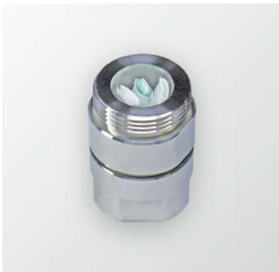
An extraction vessel enclosing sample swab
