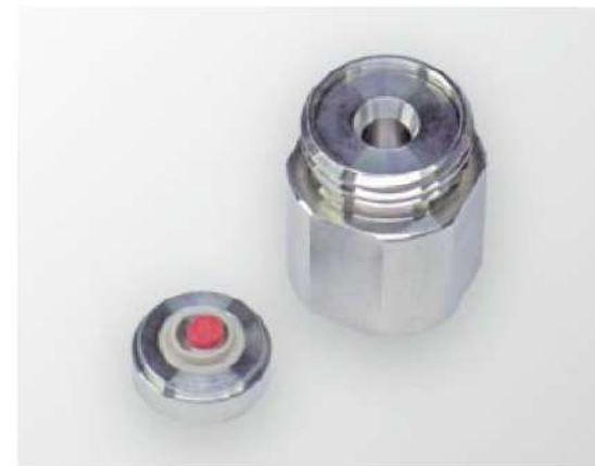
An extraction vessel for DBS
